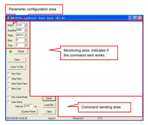
Please set the parameters of COM number, bound rate, data bit, stop bit and the parity bit correctly, then the RS232 commands can be sent in Command Sending Area.
